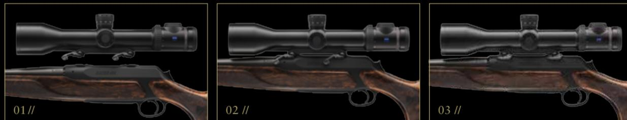
Good things come in threes: The SUM mounts effortlessly onto the S404. 01 // Tip the scope to the side so that the crossbars of the mount engage the milled slots in the receiver. 02 // Push the scope toward the muzzle and lock the rear lever. 03 // Lock the front lever.
