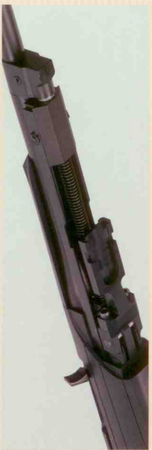
Self-cleaning: the unique gas system of the SR1.
